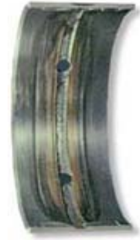
Bearing Wear caused by oil dilution
