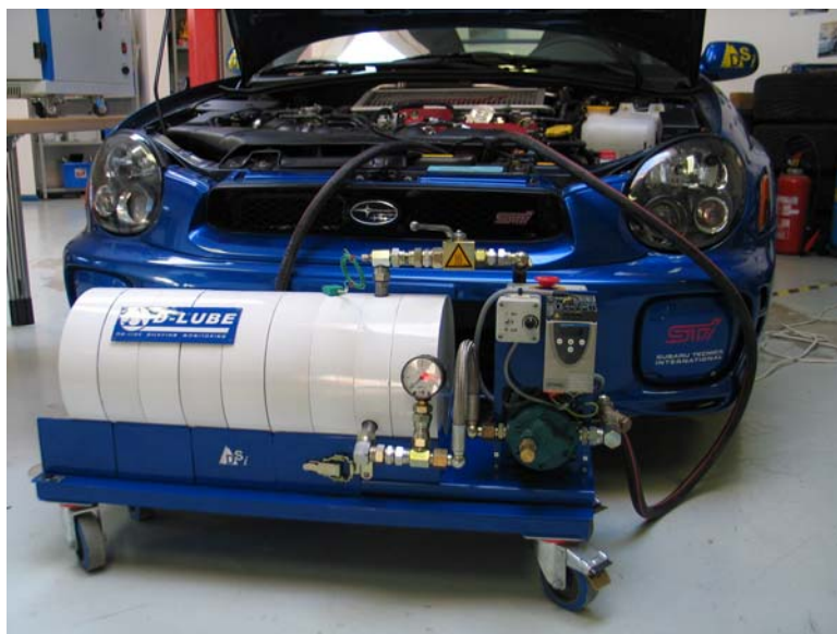
FIG.2: REAL-TIME OIL DILUTION MEASURING DEVICE
