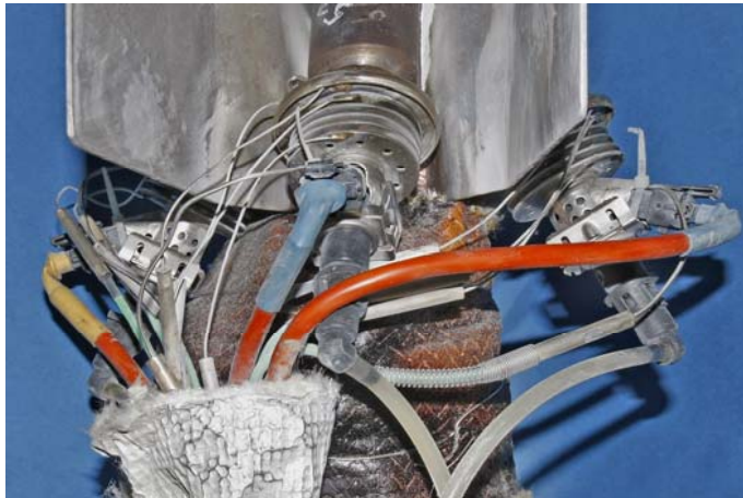
Equipment of Exhaust Gas System with several DeNox Injectors
