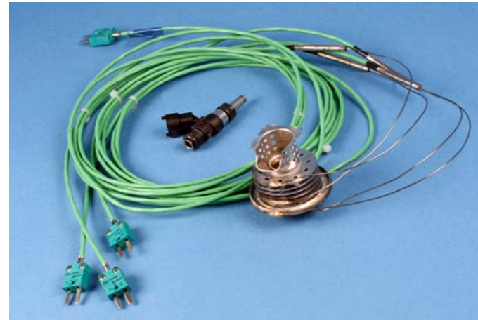
Cooling Element of a DeNox Injector with Thermocouples
