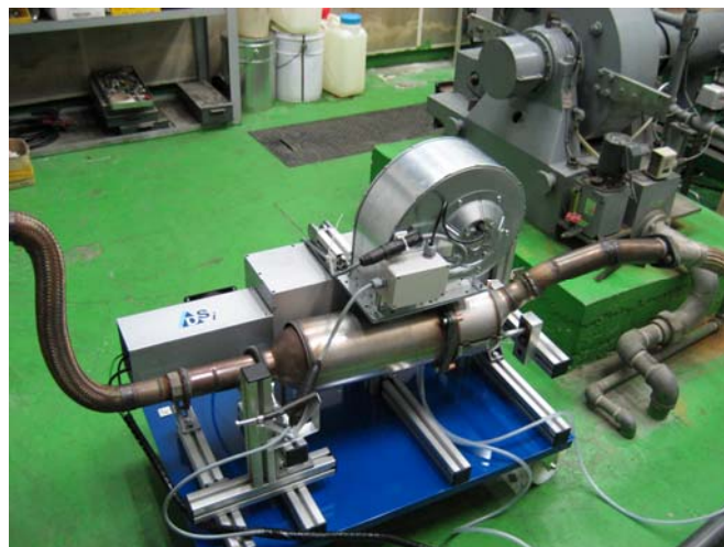
REAL-TIME OIL CONSUMPTION MEASUREMENT PROBE INSTALLED IN THE EXHAUST LINE
