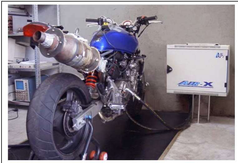
View on the sampling unit of Air-X and detail on the connecting system
